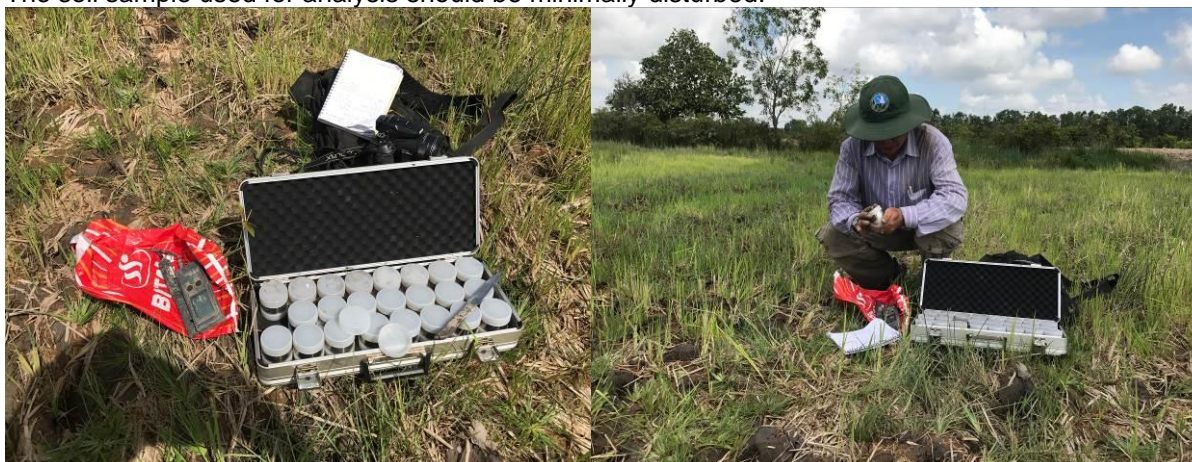
Figure 14: A specialized sampling kit used for soil bulk density analysis (Photo: Quoi, 2018).
